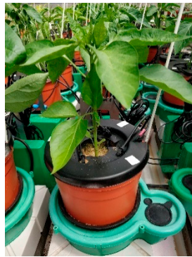
Figure 1. A pot in the greenhouse. Four drippers provided the water and nutrients, while evaporation was restricted with a plastic cover. The pot was loaded onto a green plastic container that collected a predetermined amount of drainage. The pot and plastic container were placed on a scale which is connected to Plantarray 3.0 system.
